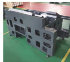
Honeycomb shape strong structure
