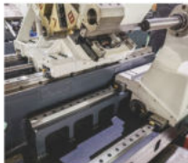
Hydraulic programmable tailstock
