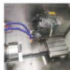
H40TC SAUTER 12T VDI30 powered tool turret
