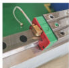
Z axis ROLLER type linear guideway
